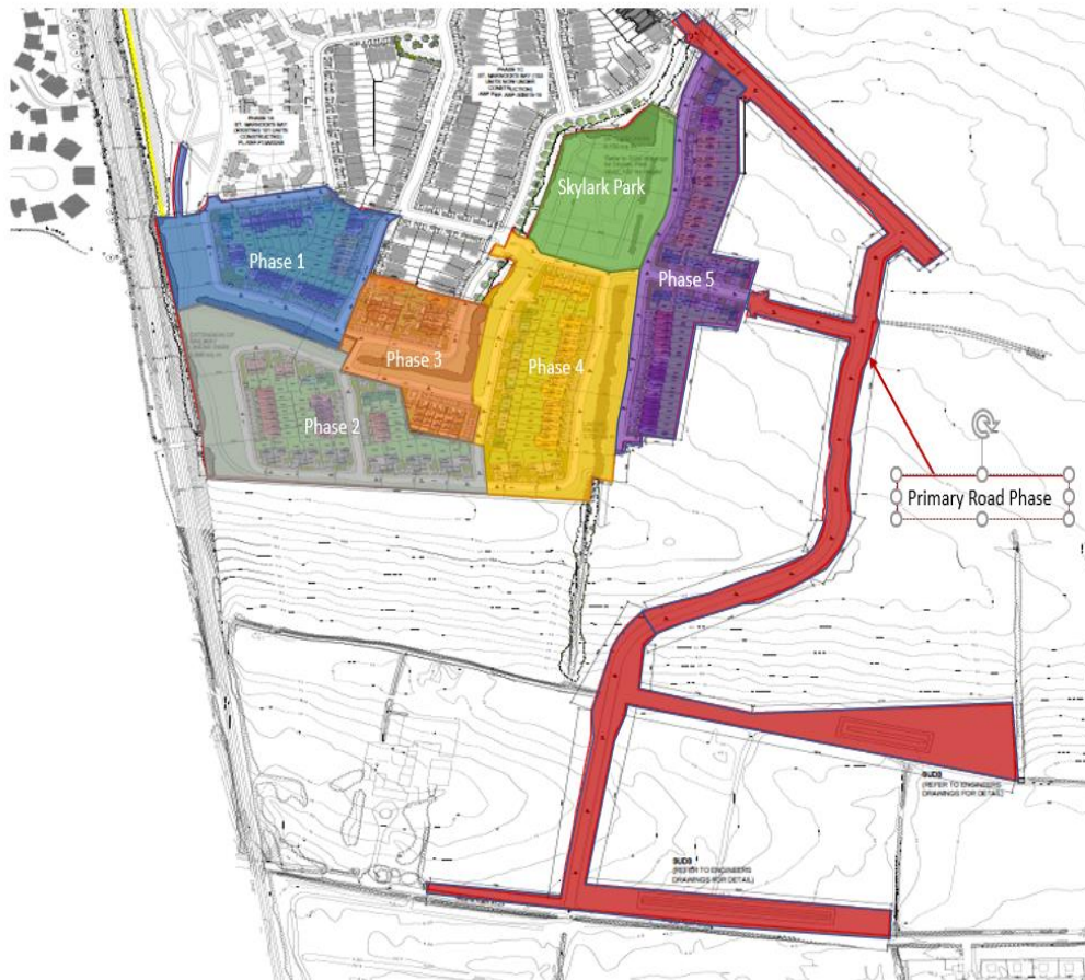
Figure 1.0: Indicative Site Construction Phasing Plan
